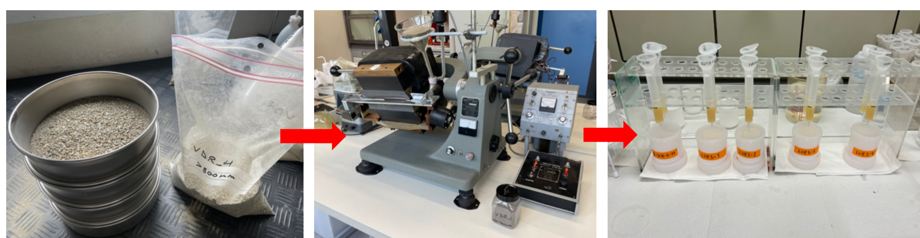
Figure 2. (A) Sieving for 250-400 μm size sediment (B) magnetic separation (C) Anion Column during chemical separation (D) Coalesced fan at Sedrun (Dieleman et al., 2018)
