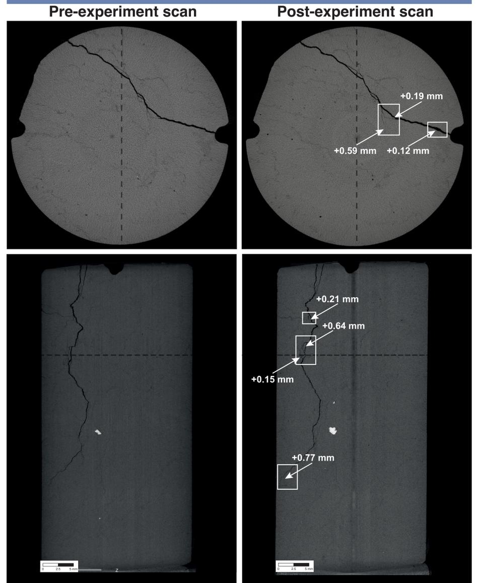
**Figure 3:** Images of the CT-Scan “Stellhorn 01”. The image’s grayscale reflects the density variations, with darker areas showing lower densities (like fractures or pores) and lighter areas denoting higher densities. The white rectangles indicate the areas of fracture propagation or widened.
