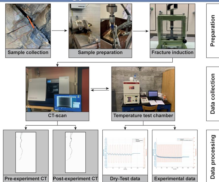
**Figure 2:** Workflow diagram for the fracture experiments
