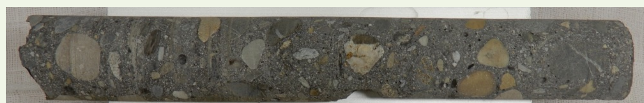
Figure 3: Drill core with a diameter of 3 cm and a length of 21 cm.
