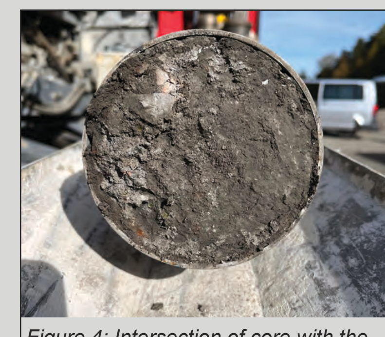
Figure 4: Intersection of core with the dark layer created by friction visible
