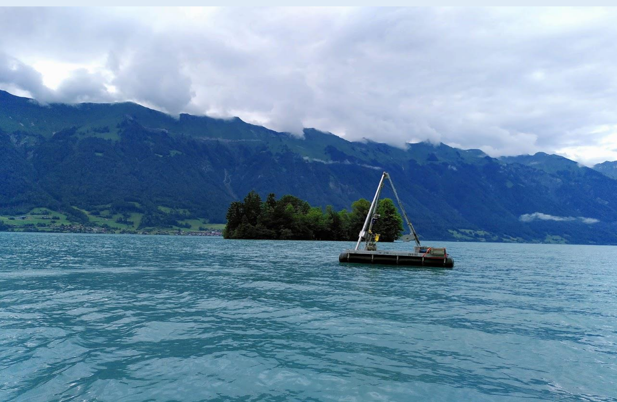
Coring platform Helvetia at the Iseltwald drill site
