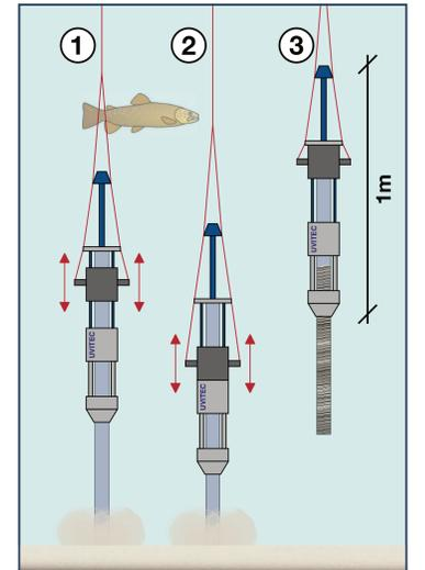
Fig. 4: Uvitec coring device, the weight (dark grey) gets pulled up by hand, releasing the weight the plastic liner plunges into the sediments
