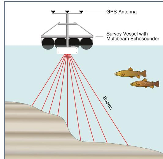
Fig. 3: Survey platform with attached Multibeam Echosounder
