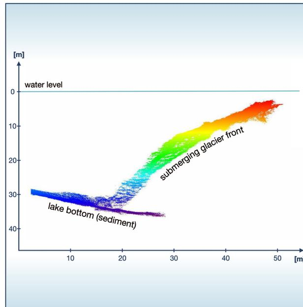
Fig. 5: Point cloud of the detected submerging glacierfront (see also Fig. 4)
